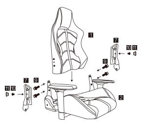
STEP 4 / 步骤四 Aim at the top of gas lift and the hole of mechanism, then put the chair body down.
